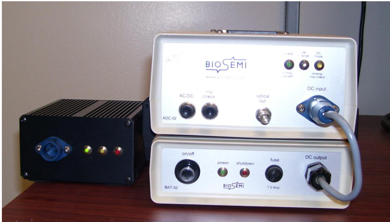
26. A front view of the EEG amplifier. On top is the Amplifier and the battery is on bottom. To the left is charging station for the battery.
