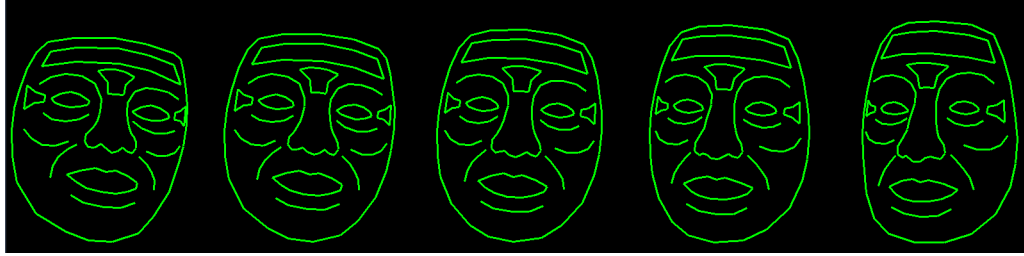
Figure 6: Example of Active Shape Models. This shape is trained across the labeled images from the database.
