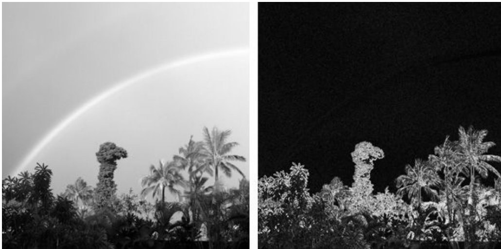
Figure 25: A sample grayscale image with parallel Sobel edge detection applied, Scaled to fit page
