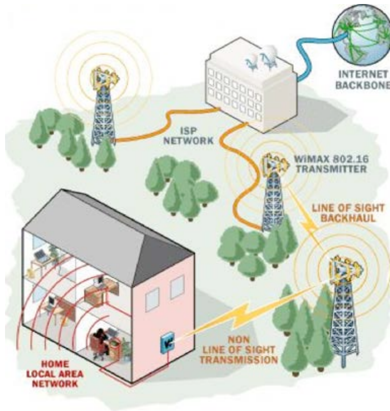
Figure 2: Components of WiMAX (source: HowStuffWorks, 2012)
