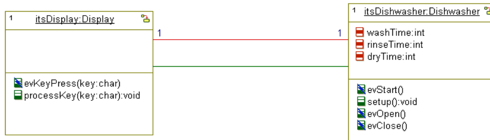
Figure 13: Object Model Diagram for the Dishwasher Project. From: IBM (2009). Java Tutorial for Rational Rhapsody. IBM Corporation. USA. Retrieved February 20, 2013, from http://publib.boulder.ibm.com/infocenter/rsdp/v1r0m0/topic/com.ibm.help.download.rhapsody.doc/pdf75/tutorialj.pdf
