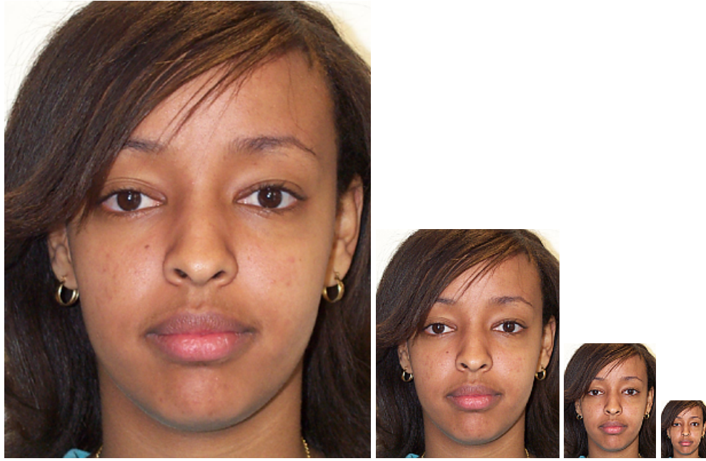
Figure 2.10: Image resolution pyramid: each level is downsampled by half of the previous structure has been located. Therefore, the image search begins at the highest pyramid level (lowest resolution) and continues until convergence has been declared, before moving on to the next level. This process is repeated until all levels have been searched. Figure 2.11 illustrates the mean profiles across three pyramid levels of a single landmark extracted from the boundary of a face. The distributions are very similar, but are not entirely the same.
