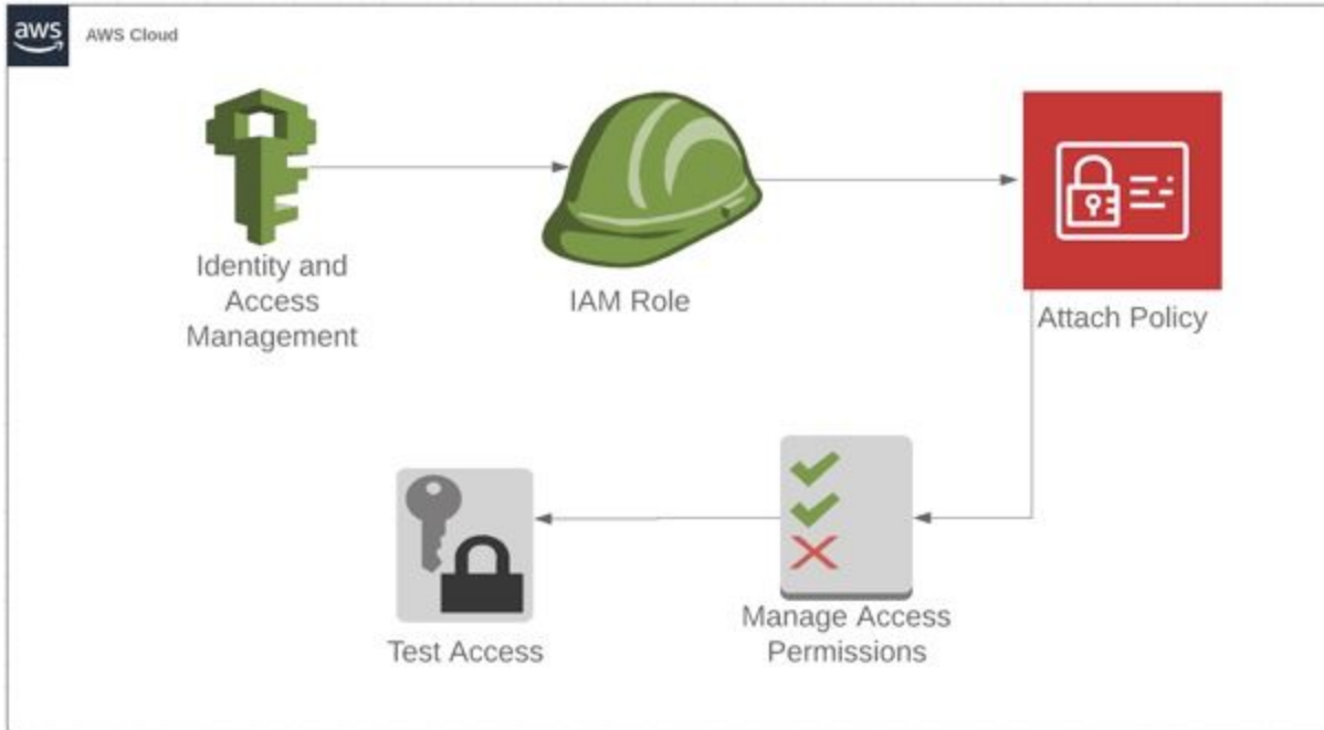
Figure 19: IAM access process has five steps. Roles are defined, policies attached, Permissions managed and access tested. IAM policy that is attached to the role is present in a JSON format
