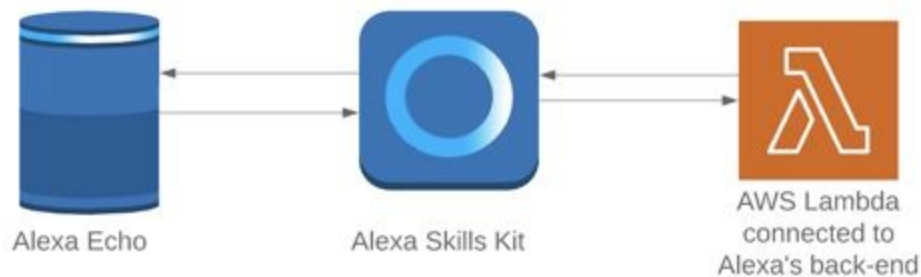
Figure 20: General Voice Only Architecture Model that uses the Developer Console as the front-end and AWS Lambda as the back-end. They are connected using the ARNs generated by Amazon.
