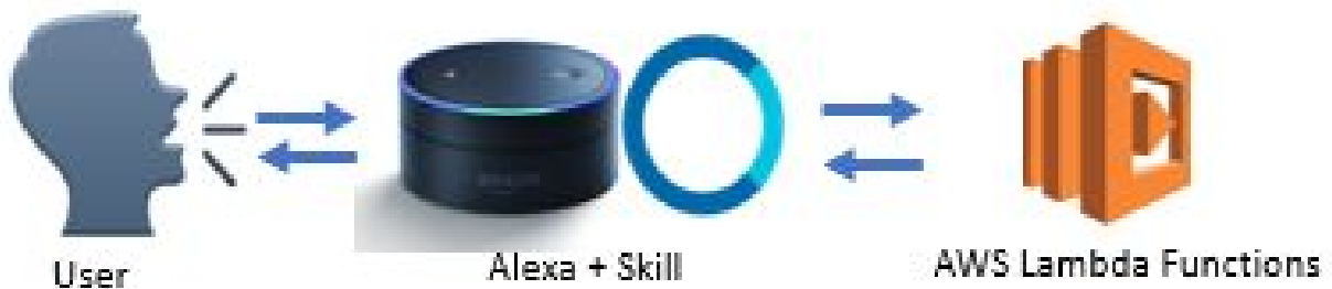
Figure 1: Architecture model of Verbiage that uses the Developer Console as the front-end and AWS Lambda as the back-end. They are connected using the ARNs generated by Amazon.
