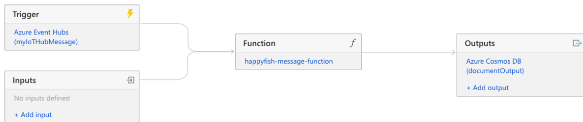
Figure 24 Dataflow from IoT Hub to Function to Cosmos DB
